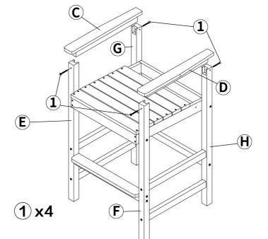
• As shown in the figure, C,E, and G are fixed together by ①, and D,F, and H are fixed together fixed together
