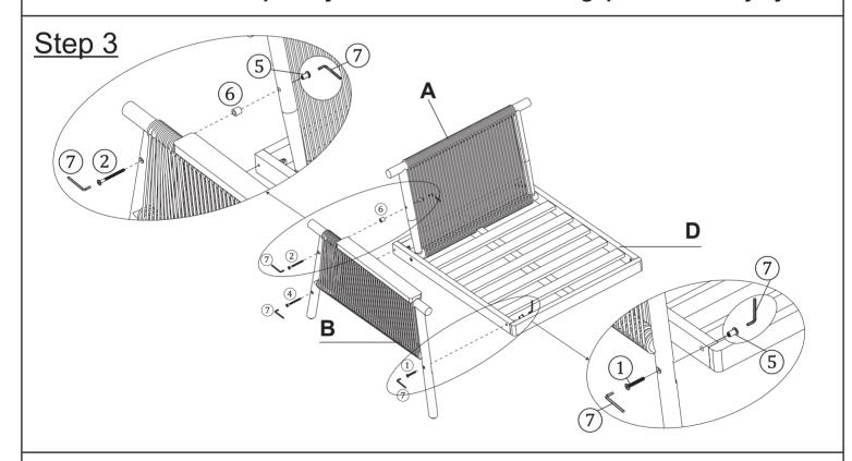
Attach the Seat Panel (D) to the Left Leg Panel (B) using Bolts (1), Screws (4), Sleeve Nut (5) and Allen Wrench (K4) (7) as shown above.
