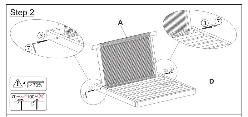
Place the Back Rest (A), Seat Panel (D) on a clean, non-marring surface. Attach Back Rest (A) to the Seat Panel (D) using Screws (3) and the Allen Wrench (K4) (7) as shown above.
