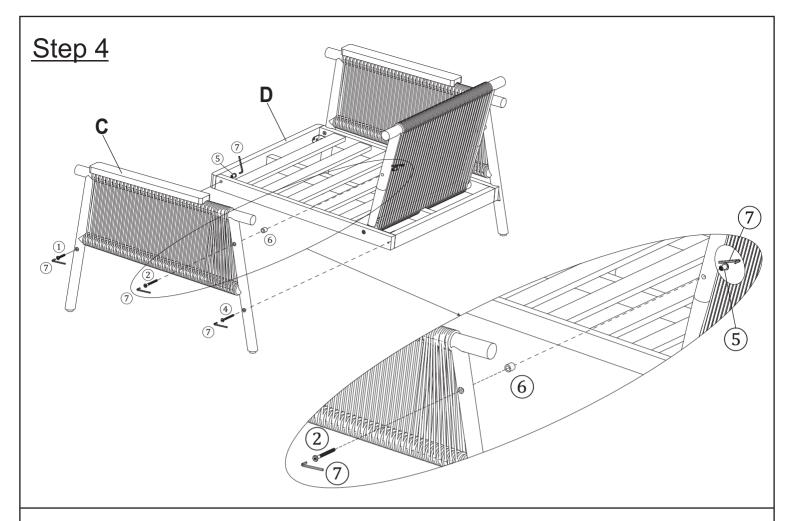
Attach the Seat Panel (D) to the Right Leg Panel (C) using Bolts (1), Screws (4), Sleeve Nut (5) and Allen Wrench (K4) (7) as shown above.
