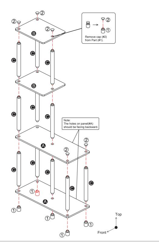
2 Top Front 3 20 20 For safety, please use the provided hardware to secure the unit onto the wall. 40 (3) Evenly Distributed **Ibs** Top Front ASSEMBLY COMPLETED
