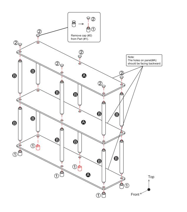
2 Top Front 3 Load Capacity Load Capacity 40 For safety, please use the provided hardware to secure the unit onto the wall. lbs 40 Evenly Distributed lbs Тор ASSEMBLY COMPLETED Front
