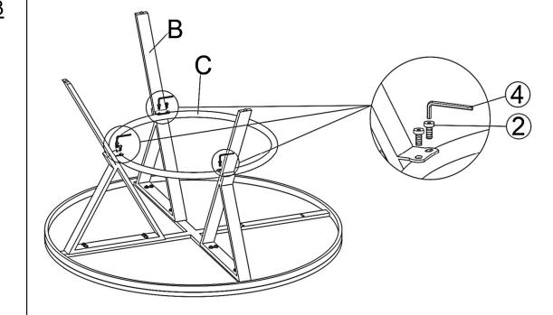
Attach the Table Stretcher(C) to the Table Lge(B) using Short Bolt(②) with Allen Wrench(④),as shown above.
