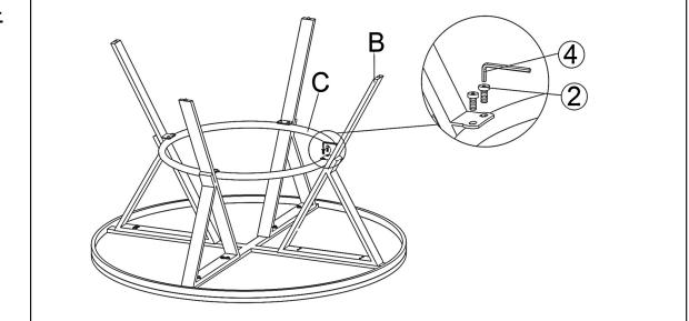
Align the hole of Fourth Table Leg (B) into the Table Stretcher (C). Attach the Fourth Table Leg (B) to the Table Stretcher (C) using Short Bolt (②) with Allen Wrench (④).
