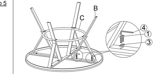
Align the hole of Fourth Table Leg (B) into the Table Top (A). Attach the Fourth Table Leg (B) to the Table Top (A) using Long Bolt (①), Flat Washer (③) with Allen Wrench (④).
