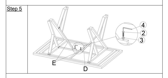
Align the hole of Table Support(E) into the Table Stretcher(D), attach Table Support(E) to the Table Stretcher(E) using Long Bolt(②), Flat Washer(③) with Allen Wrench(④).
