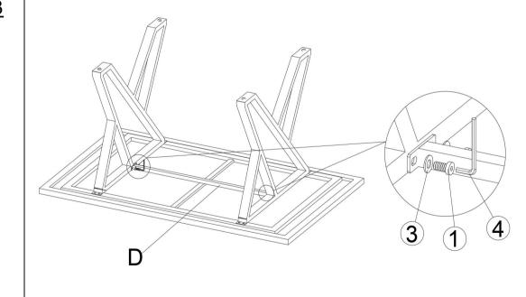
Attach the Table Stretcher(D) to the Left Leg (B) and Right Leg (C) using Short Bolt(①), Flat Washer(③) with Allen Wrench (④).
