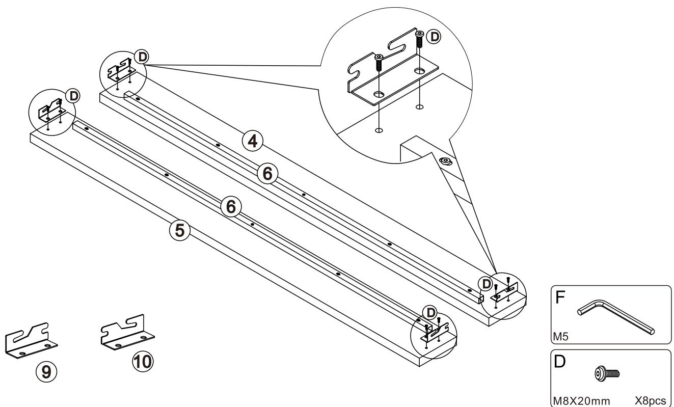
Attach the Hinge (⑨/⑩) to Side rail (④/ ⑤) with Bolts (⑪) by using Allen Wrench (⑫) .
