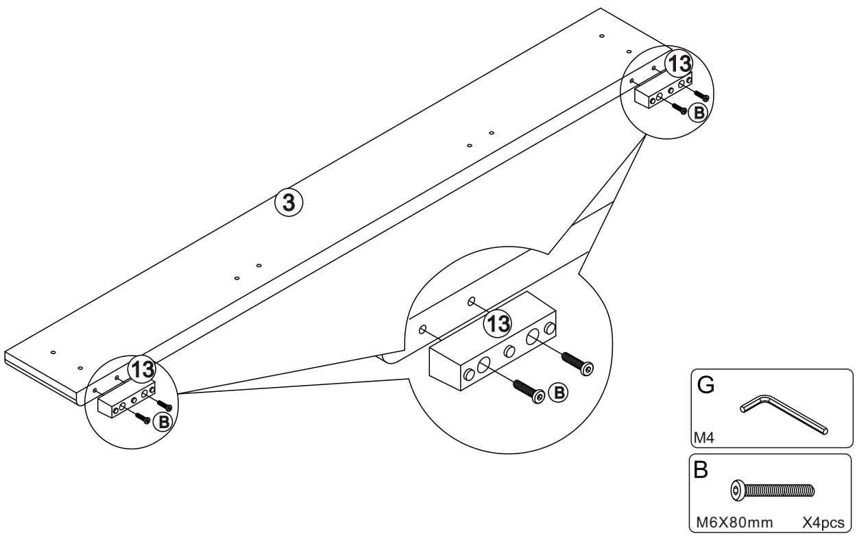
Attach Bed legs(⑬)to Footboard(③) with Bolts(⑧ ) by using Allen Wrench(⑩) .
