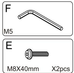
Attach the Center support bar (7) to Center support bar fittings (11) with Bolts (E) by using Allen Wrench (F).
