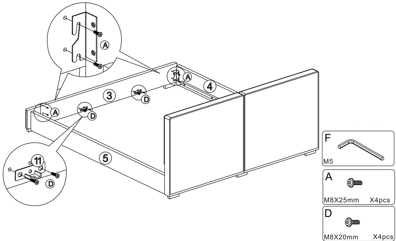
Attach the Side rail (④/⑤) and Center support bar fittings (⑪) to Footboard (③) with Hinge (⑨/⑩) and Bolts (Ⓐ/Ⓓ) by using Allen Wrench (Ⓕ).
