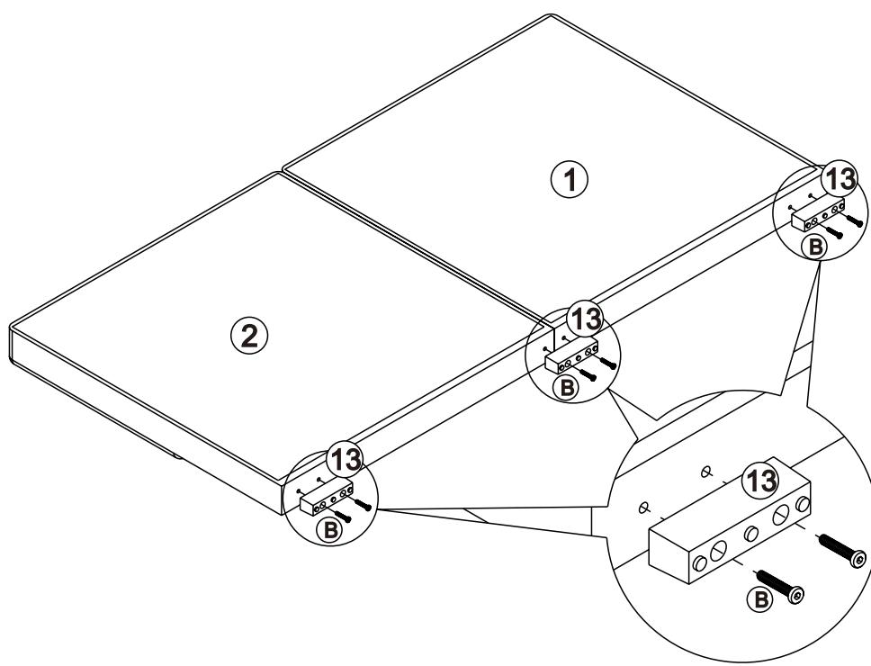
Attach the Bed legs (⑬) to Headboard (①/②) with Bolts (Ⓑ) by using Allen Wrench ( Ⓛ ).
