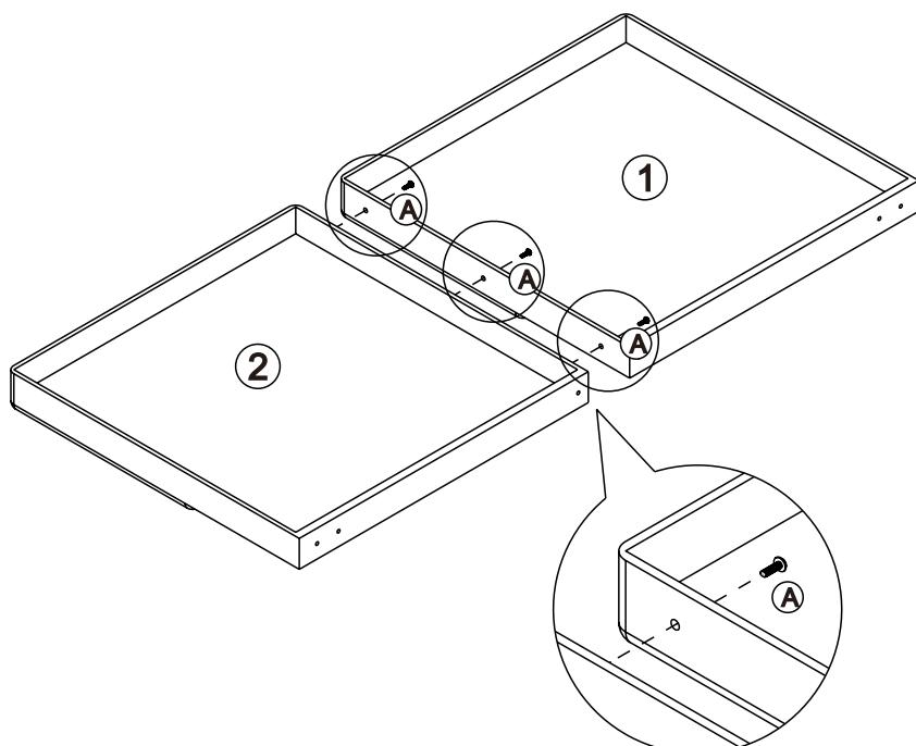
Attach the Headboard (①) to Headboard (②) With Bolts (Ⓐ ) by using Allen Wrench ( Ⓛ ) .
