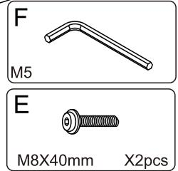
Attach the Center support bar (7) to Center support bar fittings (11) with Bolts (E) by using Allen Wrench (F).
