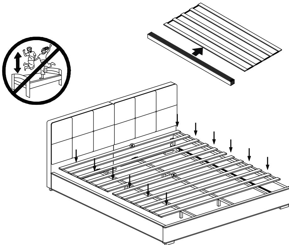
Attach the Slats (⑧) to Side rail (④/⑤) with by using magic tape.
