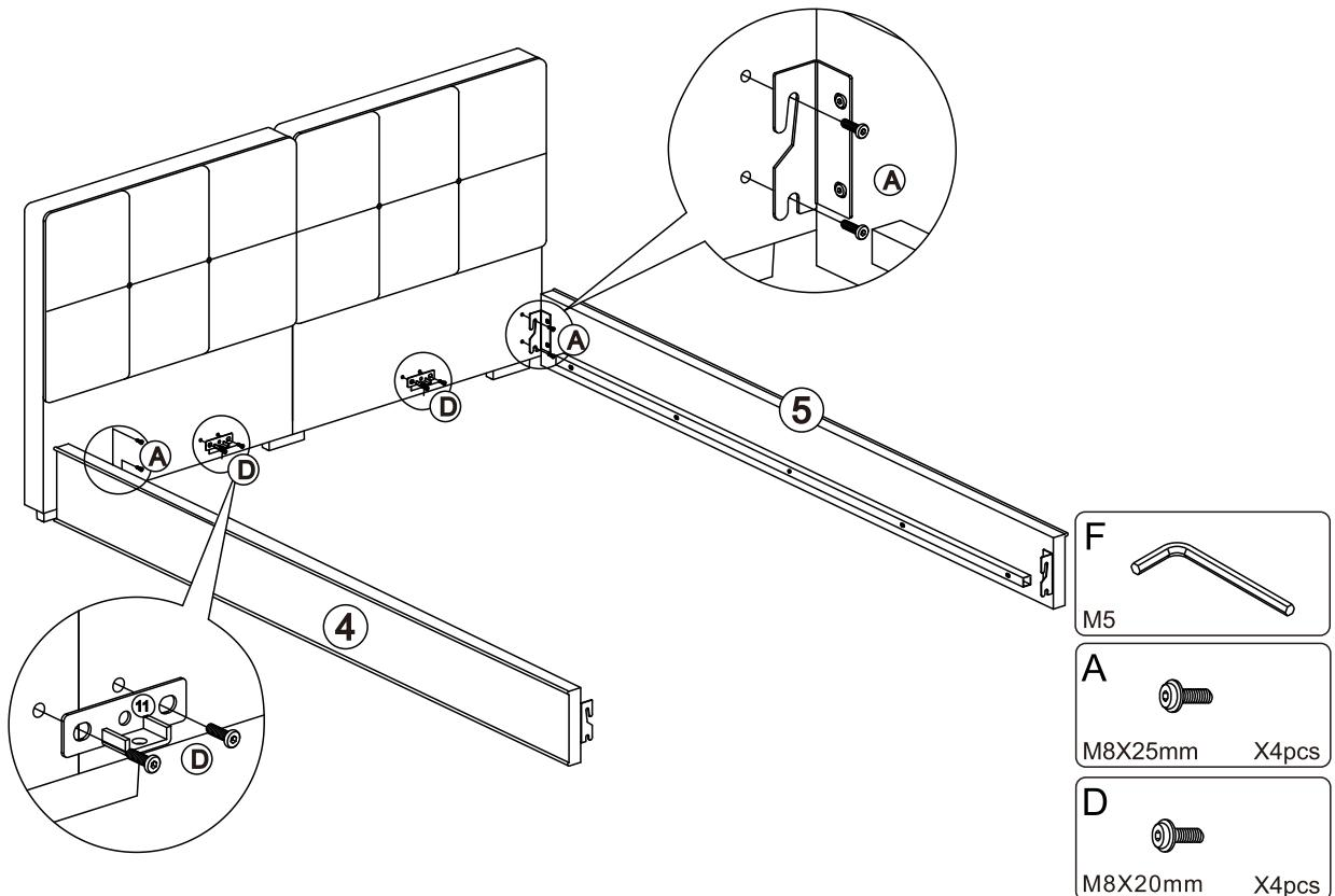
Attach the Side rail (④/⑤) and Center support bar fittings (⑪) to Headboard (①/②) with Hinge (⑨/⑩) and Bolts (Ⓐ/Ⓓ) by using Allen Wrench (⑫).
