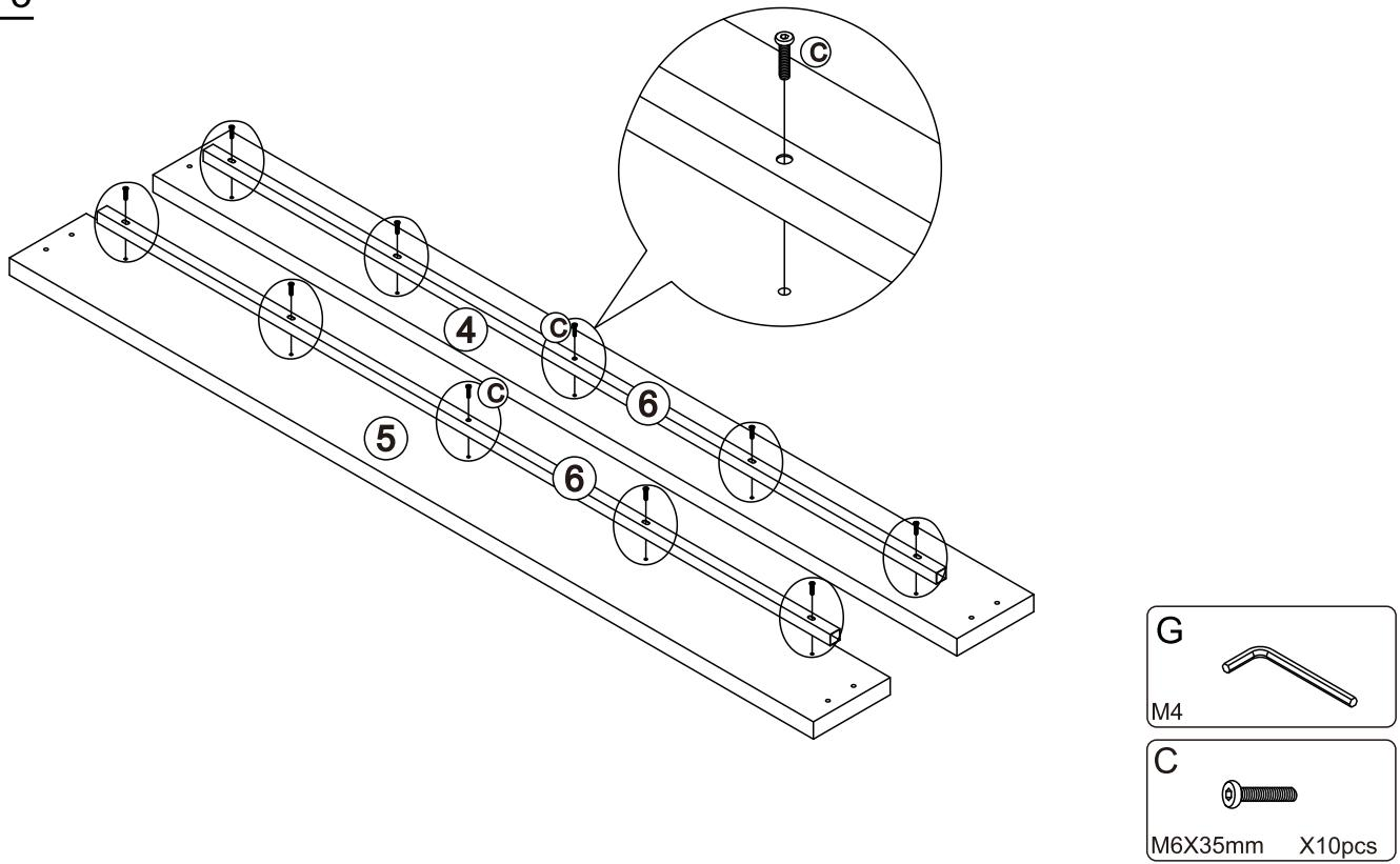
Attach the Side rails support bar (⑥) to Side rail (④ / ⑤) with Bolts(⑦)by using Allen Wrench (⑧).
