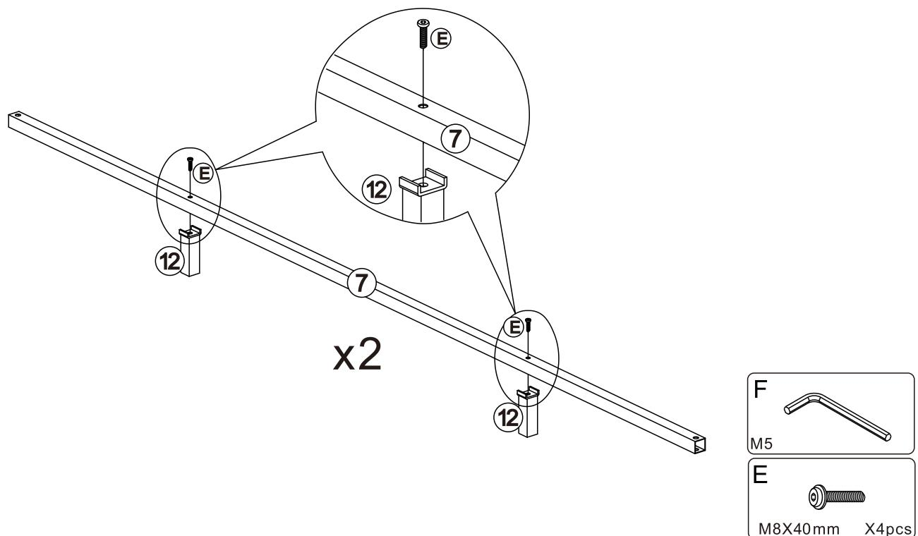
Attach the Center support bar (⑦) to Middle support legs( ⑫) with Bolts (Ⓔ) by using Allen Wrench (Ⓕ).
