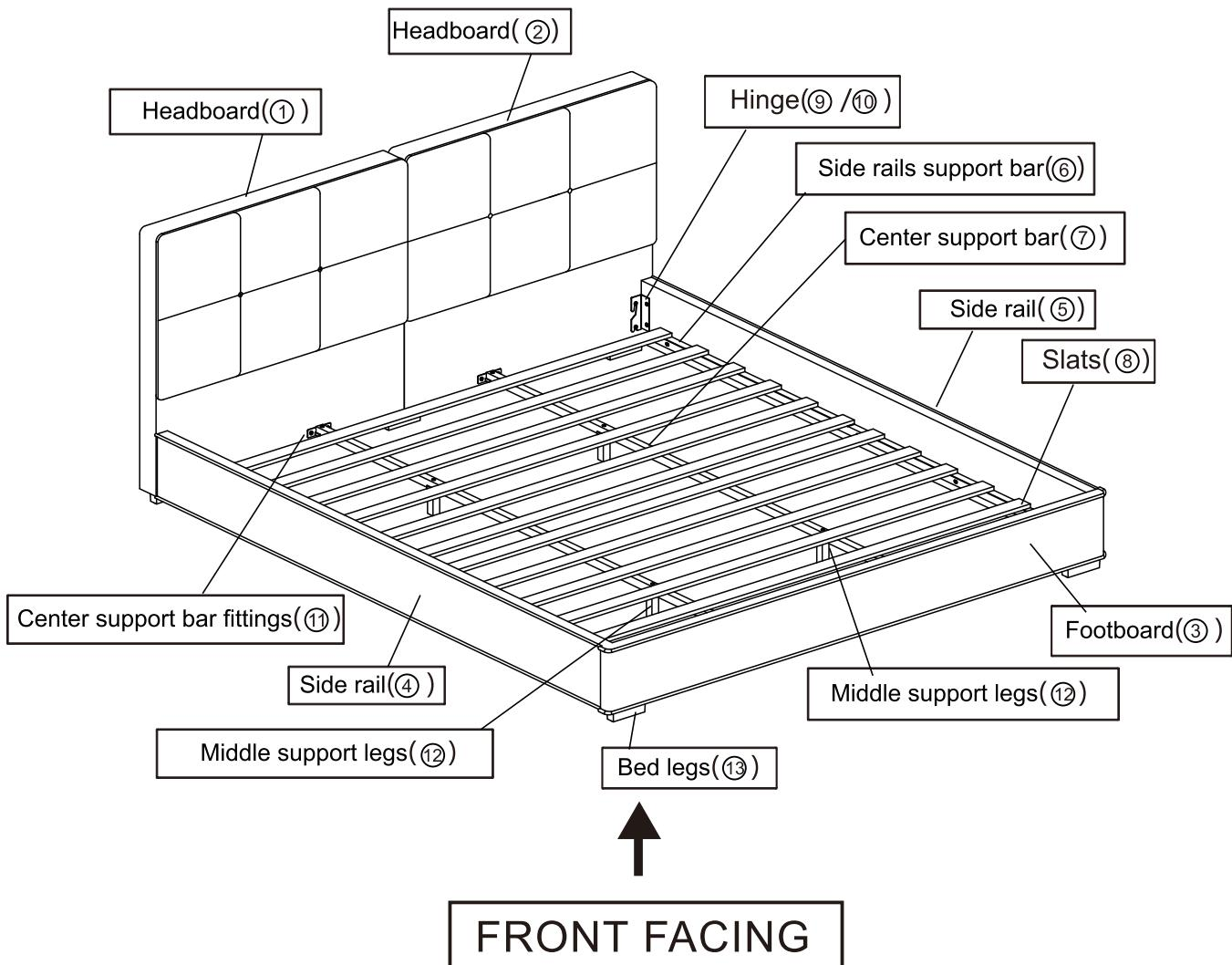
This Bed have multiple parts and may require up to 60 minutes to assemble. To give you an overview of the Bed parts, the above picture is to help you put the various parts into perspective. Please read through the instructions below to familiarise yourself with the parts and steps before assembly.
