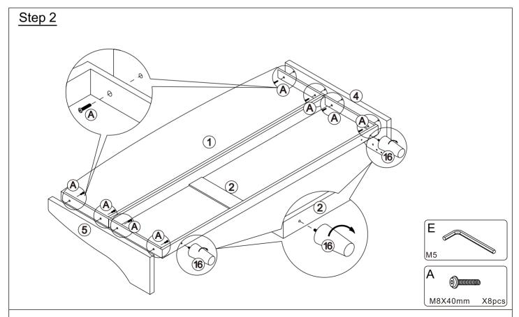
Attach the Side flank (4/5) and Bed leg(6) to Headboard (1/2) with Bolts (A) by using Allen Wrench(E).
