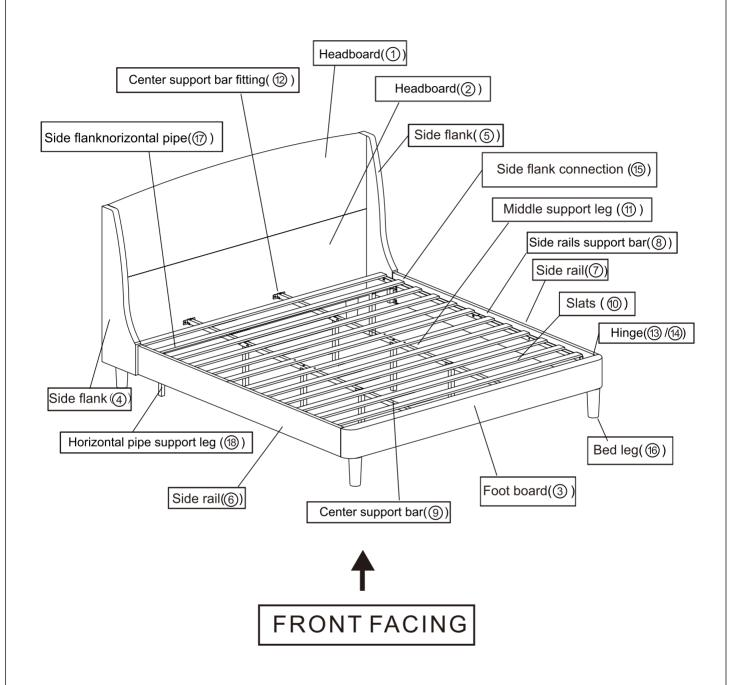
This Bed have multiple parts and may require up to 60 minutes to assemble. To give you an overview of the Bed parts, the above picture is to help you put the various parts into perspective. Please read through the instructions below to familiarise yourself with the parts and steps before assembly. Note: It is recommended that you have an adult partner to assist during the entire assembly process.
