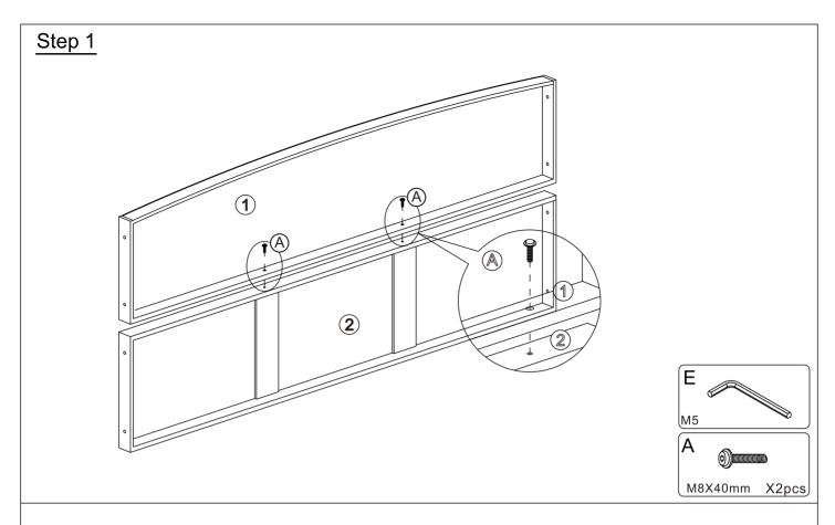
Attach the Headboard (1) to Headboard (2) with Bolts (A) by using Allen Wrench (E).
