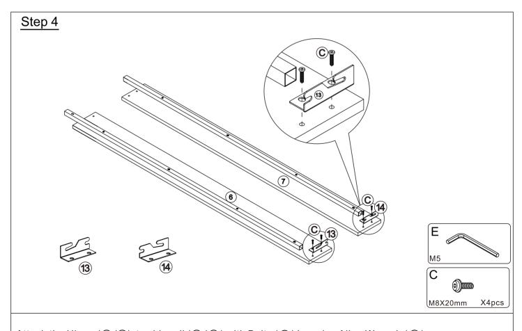
Attach the Hinge ( 3 / 4 ) to side rail ( 6 / 7 ) with Bolts ( 0 ) by using Allen Wrench ( E ) .
