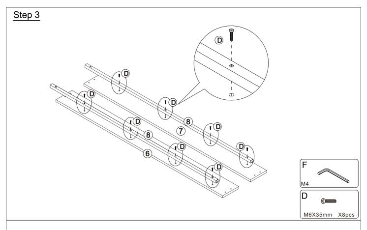
Attach the Side rails support bar (8) to side rail (6/7) with Bolts (0) by using Allen Wrench (F).
