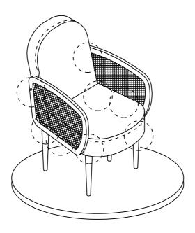
Place the chair on the flat surface and adjust the alignment and balance of the legs then , Please screw tight the steps 4, 5, 6 bolts.
