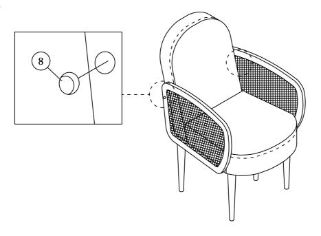
Insert and secure the hardware parts (8) to the Arm (C) and Arm (D).
