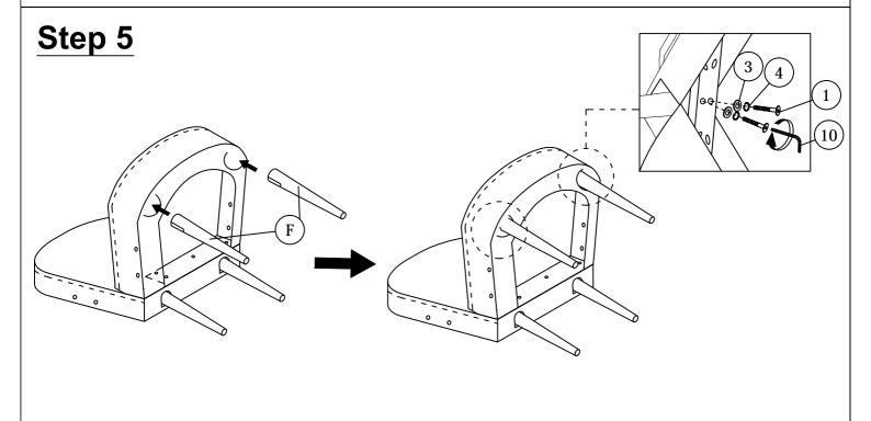
Insert and secure the Front Leg (F) to the Seat (B) using hardware parts (1),(3),(4),(10).
