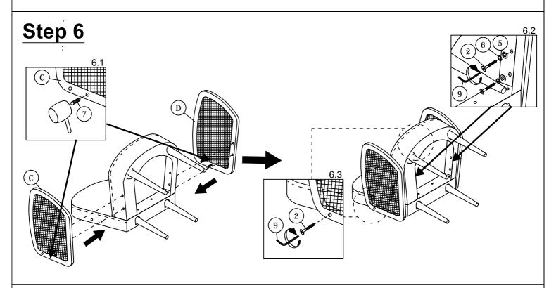
Insert and secure the Arm (C) and Arm (D) to the Back (A) and Seat (B) using hardware parts (2),(5),(6),(7),(9).
