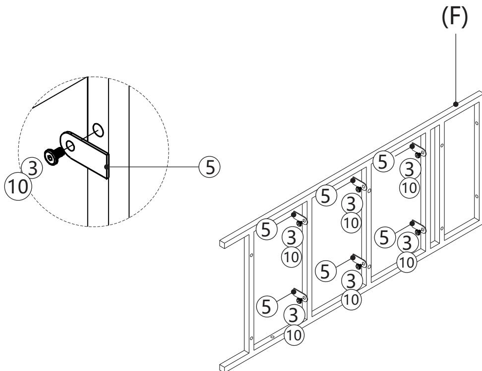
**Step 5:** Connect (F) with (A) and (B) by bolt (2) and (10).
