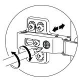
This screw can adjust the cabinet door to left or right, parallel cabinet boby with cabinet door.
