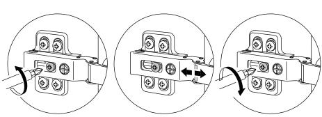
This screw can adjust the cabinet door to front or back, parallel cabinet boby with cabinet door.
