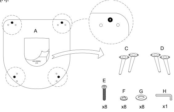
Attach the Left Leg (C) and the Right Leg (D) to the Seat (A) using Allen Bolt (E), Spring Washer (F) and Flat Washer (G) with the Allen Key (H).
