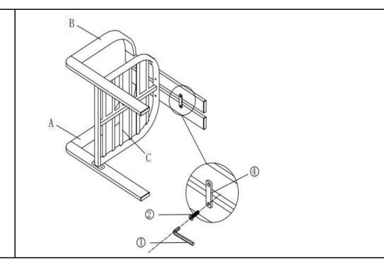
Attach the Right Armrest/Leg(B) to the Left Armrest/Leg(A) using Bolts(②) Washers(④) with the Allen Wrench(①) as shown above.
