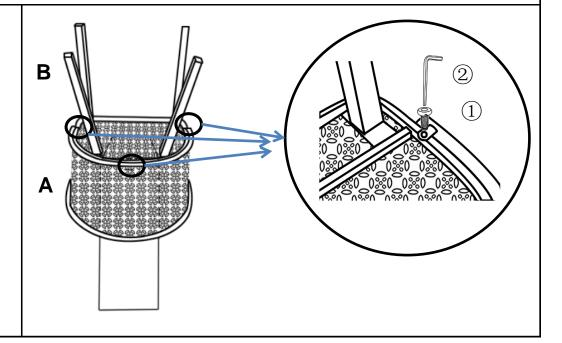
Attach Seat (B) to Backrest(A) using Bolt(①) with Allen Wrench(②). Caution: When tightening these Bolts, tighten sequentially. DO NOT tighten any screw fully and then towards the next one.
