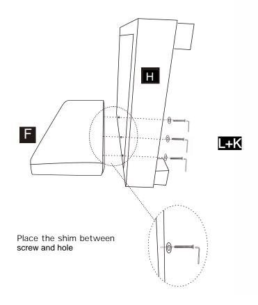
Place the frame(H) on the side as shown, and align the backrest(F) to the face of sofa frame with THREE screw holes. Make sure all three hole are aligned, then use the tools provided(Allen Key, K) to twist one screw to each hole. Twist in all four screws by 30%, make sure all the screws are able to twist, then tighten them.
