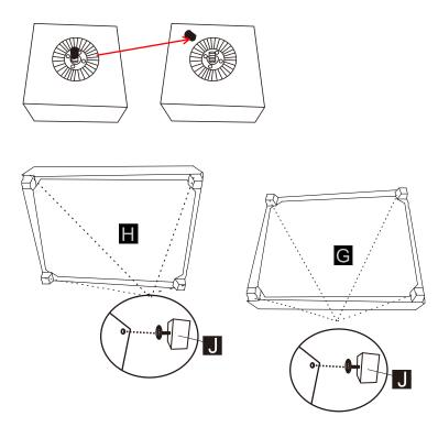
Place the wood frames(G and H) along the side as shown, and take out sofa foot(J), align the foot to each corner of the frame as shown, and gently rotate clockwise to install the wooden foot.
