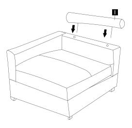
Place the headrest(I) to the top of the backrest(F) as shown, align both rods into the holes on backrest. Make sure the headrest face to the front. There are three level adjustment for the headrest.
