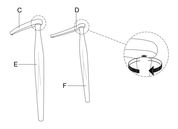
Attach the Left Front Leg (E) to the Cushion Seat (B) using JCBC Bolt (I), Lock Washer (K) and Flat Washer (L) with the Allen Key (N). Then, attach the Left Arm (C) to the Back Frame (A) using Wood Screw (M) with a screwdriver (not provided).
