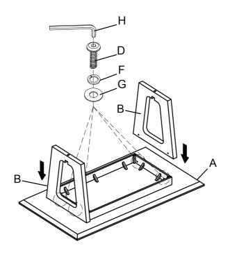
2 Attach the Stretcher (C) to the Leg (B) using Bolt (E), Lock Washer (F) and Flat Washer (G) with the Allen Key (H).
