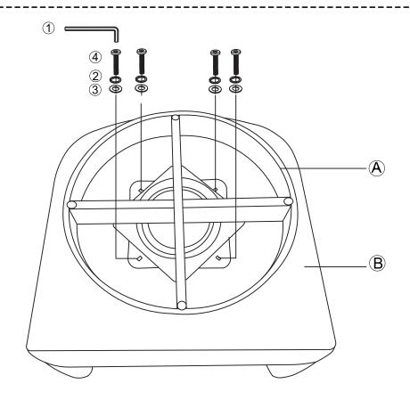
Note: Rotate the swivel plate to cross and separate the upper and lower iron plates, aligning the four holes in the lower iron plate with the four screw holes on the seat frame.
