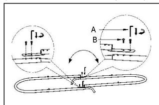
Step 1:Lay the lamp body (K) flat and secure it with allen wrench (A) and screw (B).
