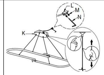
**Step 4.** Press the expansion piece and adjust the height of the lamp body(K). If the expansion piece fails, Move wire locking device(L) to the desired position and lock it with hex screw (M) and allen wrench (N).
