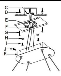
Step 2: Punch the hole and install the Wall plug (D) to the ceiling. Fix the mounting bracket (E) to the outlet box with tapping screw (G) and mounting screw (I).
