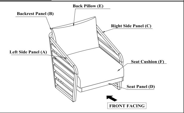
This Chair has multiple parts and may require up to 30 minutes to assemble. To give you an overview of the Chair parts, the above picture is to help you put the various parts into perspective. Please read through the instructions herebelow to familiarise yourself with the parts and steps before assembly.
