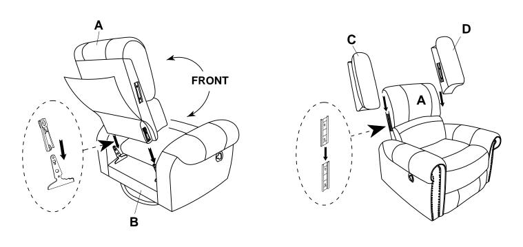
3 Use Velcro to attach the back cover to the bottom of the seat frame.
