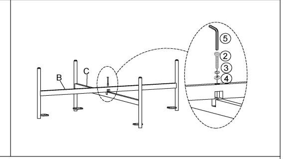
Attach Lower Leg Farme(B) to Upper Leg Farme(C) using Bolt(②), Spring Washer(③), Washing Ring(④) with Allen Wrench(⑤).
