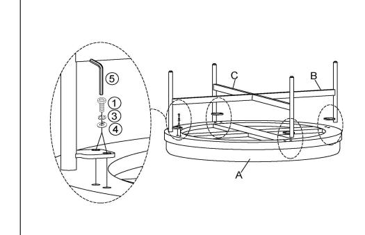
Attach Base frame Lower Leg Farme(B) and Upper Leg Farme(C) to the bottom of the Cushion(A) and using Bolt( $\bigcirc$ ), Spring Washer( $\bigcirc$ ), Washing Ring( $\bigcirc$ ) with Allen Wrench( $\bigcirc$ ).
