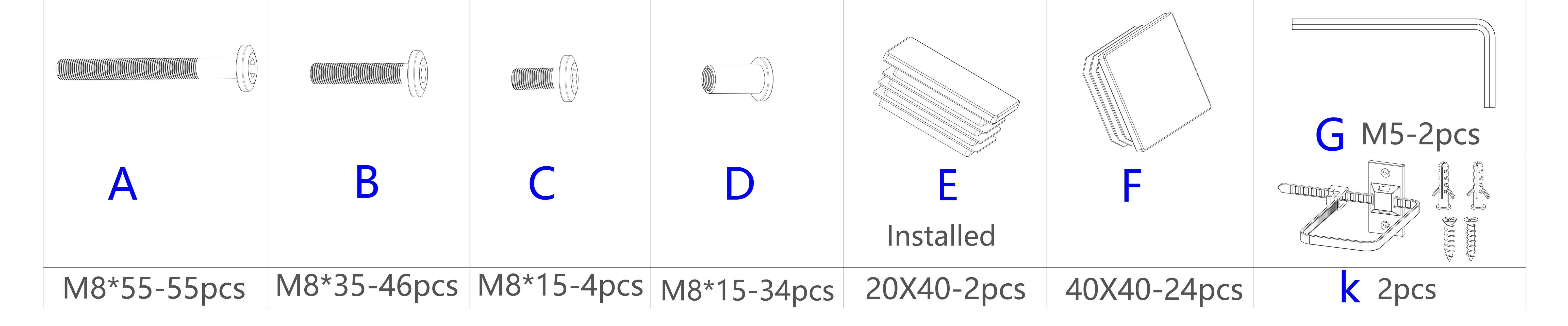
Step 1: Use hardware A, B, D, F, G to connect #3, #6, #13, #18 together. 13-1pcs 3-2pcs 6-1pcs M8\*35-3pcs M8\*15-3pcs 18-1pcs M8\*55-6pcs Step 2: Use hardware A, B, D, F, G to connect #1 and #6 together.
