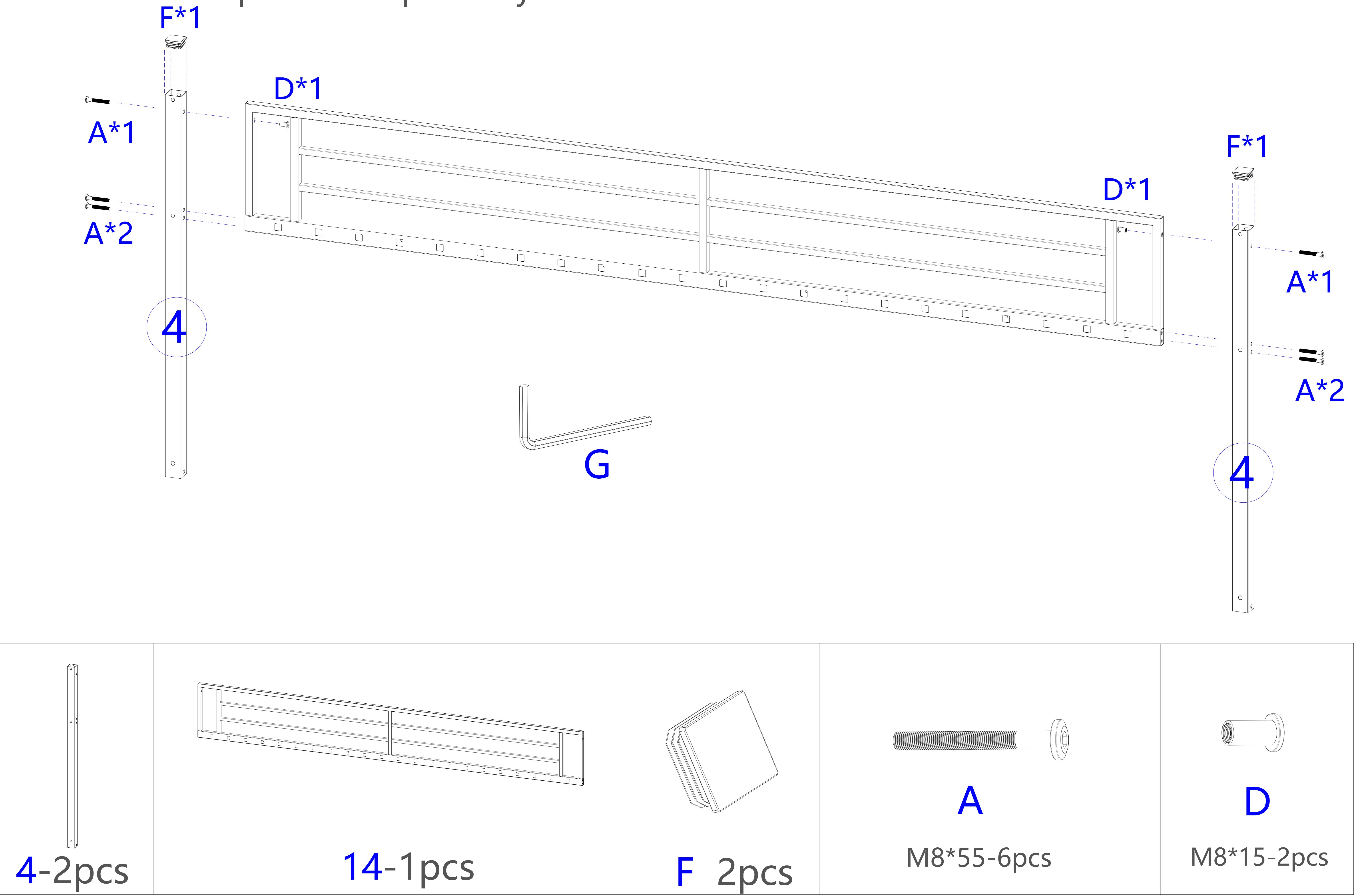
Step 10: Use B, D and G to connect the components of step 9 to the left and right
