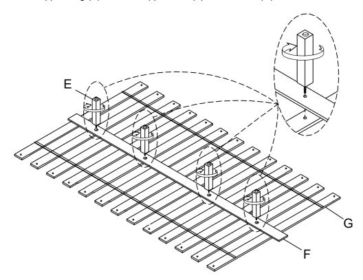
Attach the Slat (G) to the Side Rail (C) using Screw (H) with a screwdriver (not provided).
