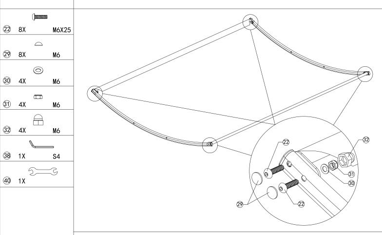
Step 7: Secure the four comers of the canopy with bolts and nuts as required (After all the bolts are assembled in place, tighten them together, finally cover the caps).
