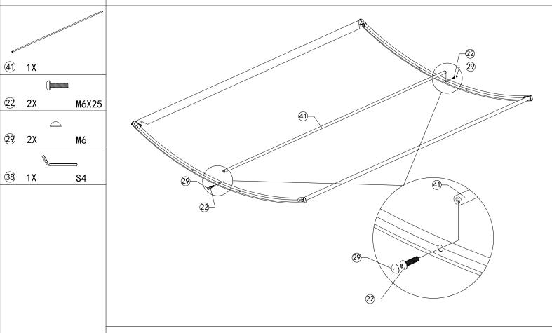
Use 2 bolts #22 to secure the middle roof support tube #41 to form the canopy frame.
