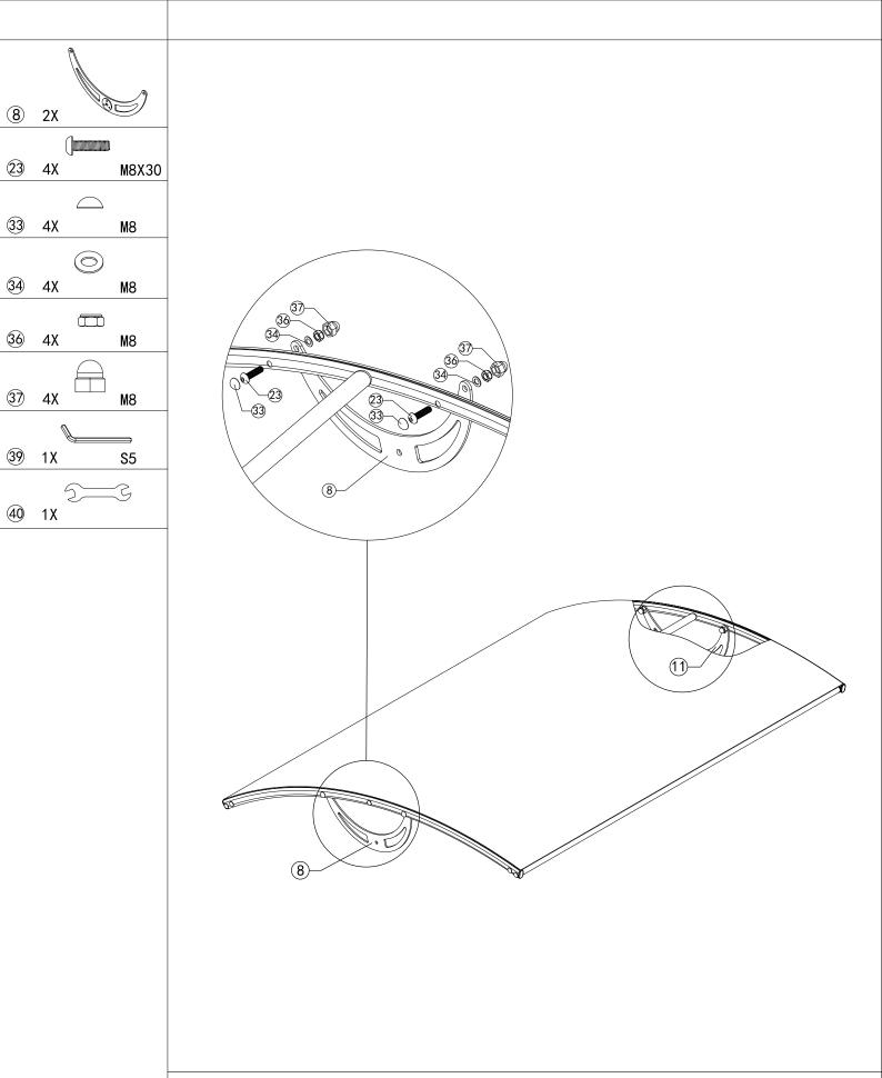
Step 8: Install Part 8 to top canopy. Align the holes and secure with bolts and nuts as required as required (After all the bolts are assembled in place, tighten them together, finally cover the caps).
