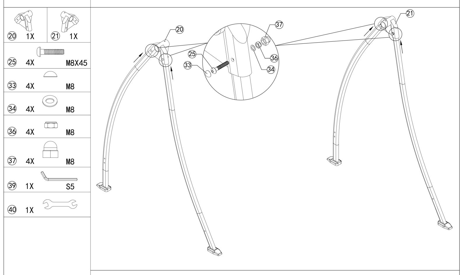
Step 2: Put the front and rear leg tubes (Part 1 is front leg tube, Part 2 is rear leg tube) into the fixator (Part 20 and Part 21) as shown, and secure with bolts and nuts as required (After all the bolts are assembled in place, tighten them together, finally cover the caps).
