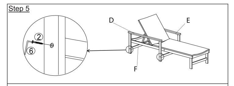
With the help from your adult partner, turn pre-assembled in step 4 right side up Affix the Left Armrest Frame(D) to Leg Support Bar(F) by using Screws(②) with Allen Wrench(⑥) as shown above.
