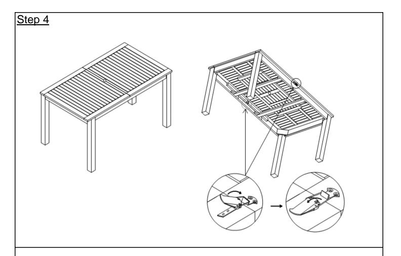
Lock the Metal Fasteners under the Table Top(A) into place as shown in the above picture.
