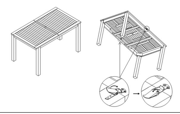
Lock the Metal Fasteners under the Table Top(A) into place as shown in the above picture. Your Table is retracted and is now ready for use.
