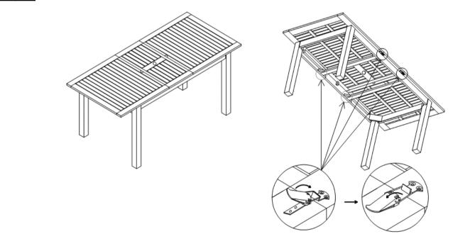
Lock the Metal Fasteners under the Table Top to lock the Expansion Board of Table Top(C) into place as shown in the above picture.
