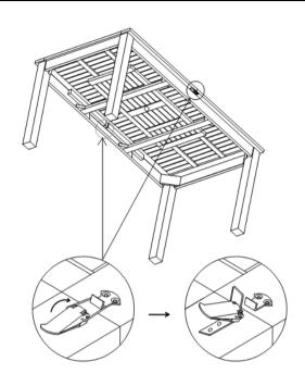
Unlock the Metal Fasteners.
