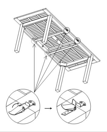
Unlock the Metal Fasteners.
