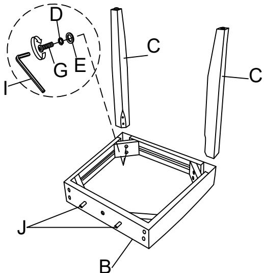
Take the Allen Key, and turn the bolts until the legs are secure.
