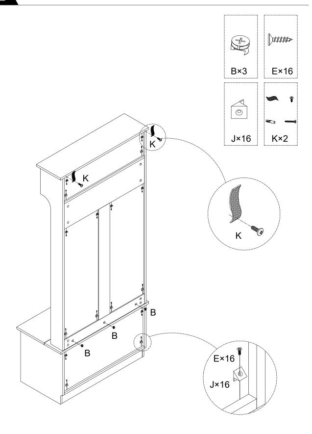
Be careful! This product must be installed to prevent dumping and fixed on the wall before it can be used! D×27 K×2 DD ①<sub>x2</sub>  $\mathbf{WALL}_{_{\perp}}$ drilling hole Ø6x30mm (II) x2 WALL III) x2 Using Cover-up Sticker D \*27 to
