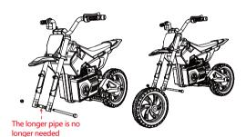
Put the front wheel on the designated position on both sides of a short shaft tube and insert the front shaft in turn, and tighten the nuts
