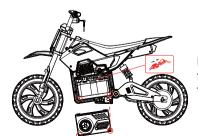
Remove the two screws first, remove the shell for use, insert the red terminal, and then install the shell, screw on
