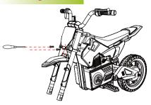
Remove the fixing screws first, then align the front tile with the hole on the car body, and screw on two screws
