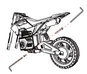
Remove the cable tie tied to the rear wheel, align the shock absorption with the hole, insert it with one long screw and one short screw, and tighten it with two Allen wrenches
