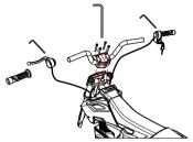
The handlebars are aligned with the body, fixed with four screws, and tightened with the hexagon, so that the left side of the handlebar can be threaded through the start brake and handle cover, the right side of the handlebar can be threaded into the turn handle, and the hand brake and turn handle can be fixed with the hexagon
