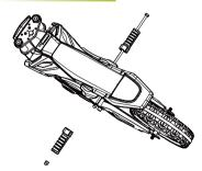
Install the foot left and right in the corresponding position, the shaft aligns with the foot through the left side, and screw on the nut
