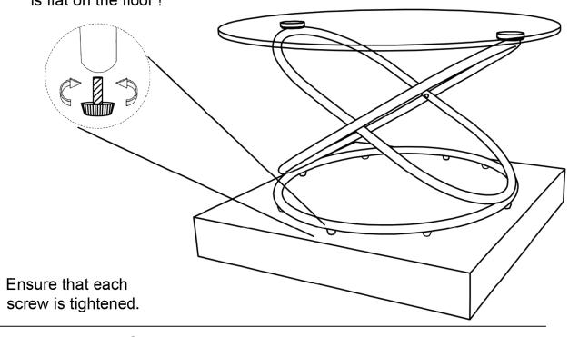
Additional Note About Safety: Bolts may loosen during normal everyday use. They should be periodically inspected and tightened to prevent damage or injury. Always check to be sure that all hardware is kept tightened. Thank you for your purchase.
