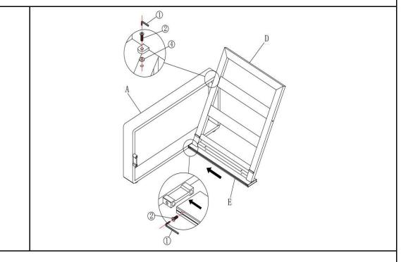
Attach Backrest (D) to Left Armrest (A) using Bolt(②) and Washer (④) with Allen Wrench (①) as shown above.
