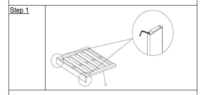
Open the carton and place all parts on a clean, non-marring surface. As shown in the figure, use Allen Wrench(①) to lift out the tube plug in Seat(C). If necessary, keep the plastic plug for repackaging.
