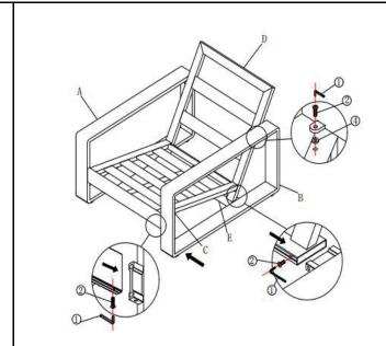
Insert the location dowel of Right Armrest (B) to the Part (C, E).
