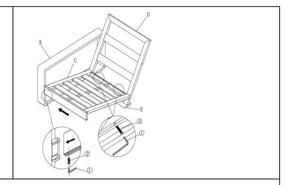
Attach the Seat (C) to Left Armrest (A), using Bolts(②) with Allen wrench (①) as shown above.
