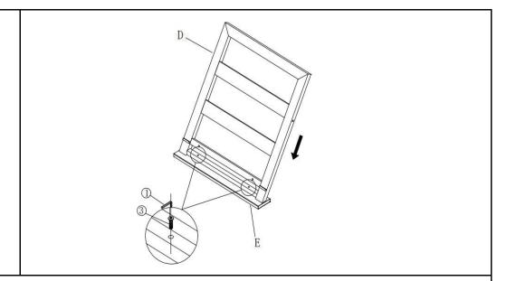
Attach the Seat (D) to Support Bar (E) using Bolt (③) with Allen Wrench (①) as shown above.
