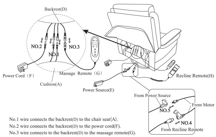
No.4 wire connects the motor's wire from the right armrest to the Recline Remote(H).
