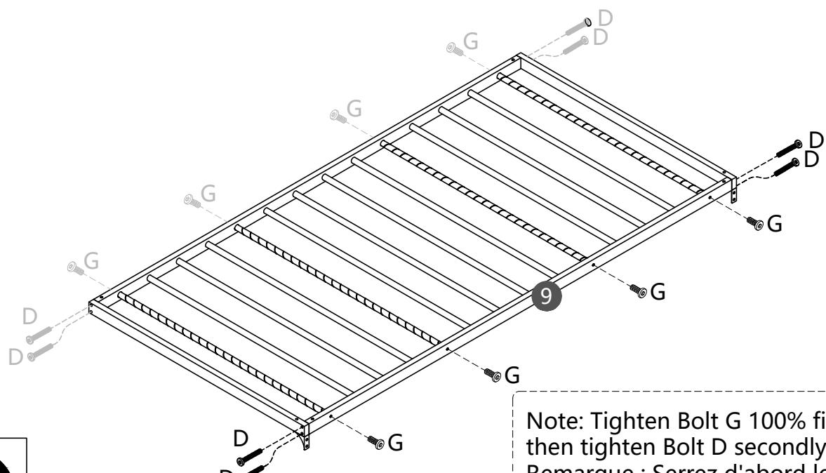
Note: Tighten Bolt G 100% firstly, then tighten Bolt D secondly.
