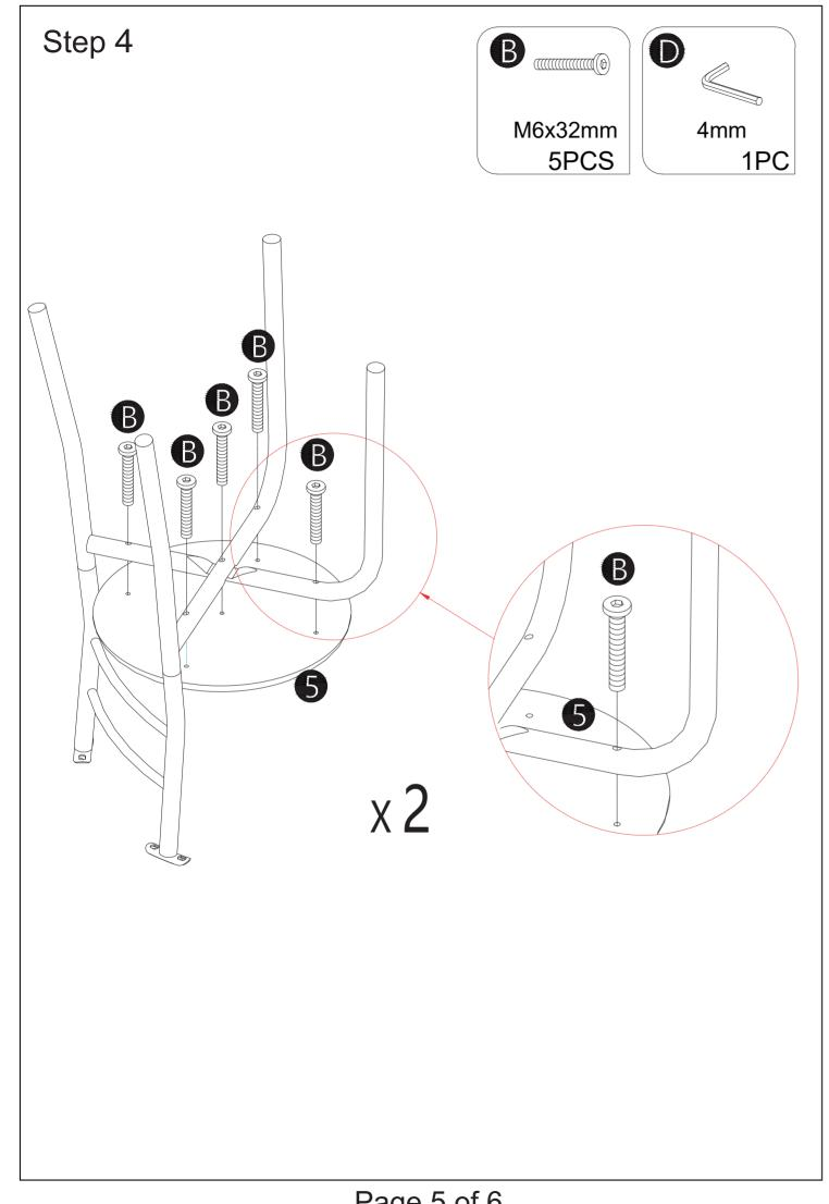
Components 2 1 1 2 670×670mm 735×620mm 3 5 2 2 573×38mm Ø360×15mm 2 2 6 7 490×120mm 356×308mm 2 2 8 9 530×473mm 530×473mm Screws & Tools A 16 **B** 14 M6x12mm M6x32mm 0 D 8 1 M6x45mm 4mm
