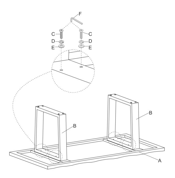
Stand the table upright and fully tighten all bolts at this step. If the table wobbles slightly, adjust the leveler on the bottom of the Table Base (B) until the table is stabilized.
