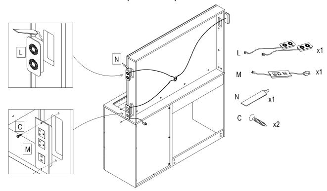
Note: ①If the speaker is not exactly embedded in the notch, glue is neccessary to fix it.
