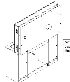
Note: Firstly drag the power cable out from the gap and then fix the mirror backboard.
