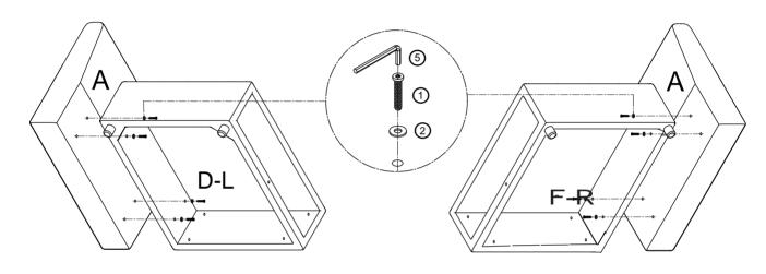
Slip over using to connect A to D-L and A to F-R.
