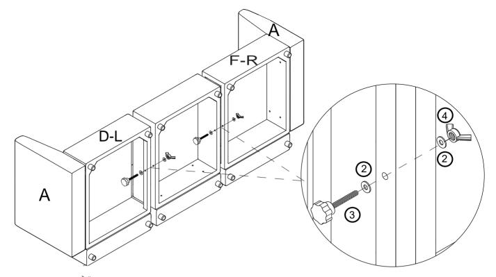
Slip over through the connection holes of the two frames, then slip another over it, and secure it with hardware.
