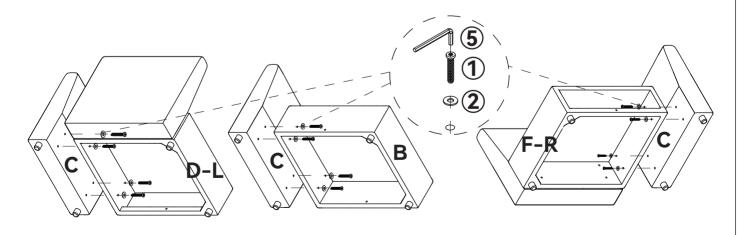
Slip over using to connect C to D-L and B to F-R.
