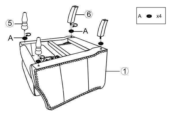
When installing the back legs, ensure that the slope is facing backwards.
