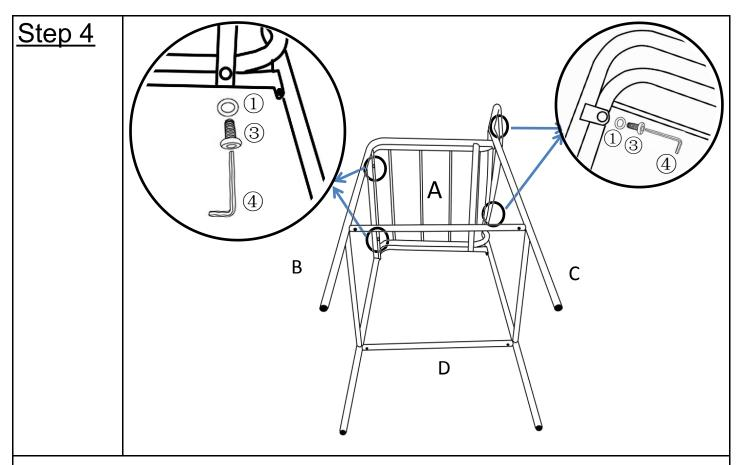
Attach Seat with backrest(A) to pre-assembled Seat frame with front legs(B) using Bolts(③) and Flat Washer Rings(①)with Allen Wrench(④). **Loosely tighten Bolts.**
