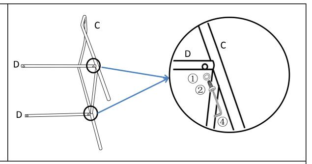
Attach Connect bar(Left&Right)(D) to Back legs with backrest frame(C) using Bolts(2) and Flat Washer Rings(1) with Allen Wrench(4). Loosely tighten Bolts.
