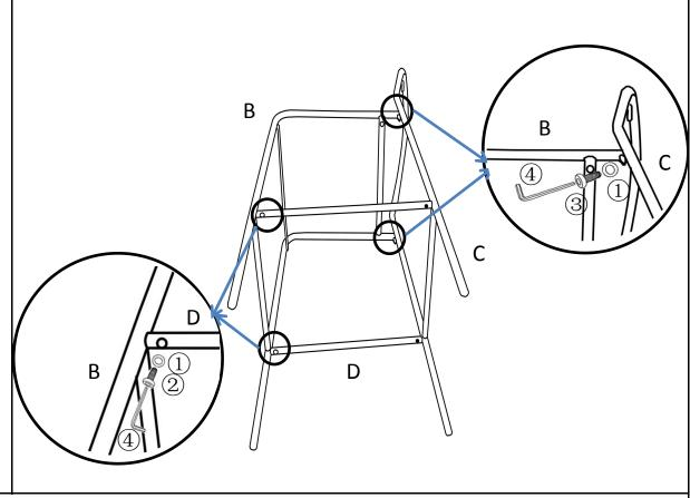
Attach Seat frame with front legs(B) to pre-assembled Back legs with backrest frame(C) and Connect bar(Left&Right)(D) using Bolts(②③) and Flat Washer Rings(①)with Allen Wrench(④). Loosely tighten Bolts.
