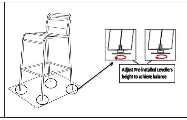
Adjust the Pre-installed Levellers at the base of the Legs until the Barstool is level to the ground.
