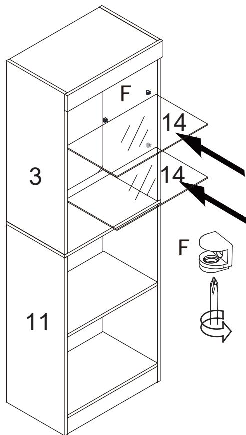
Please use a screwdriver to screw the bottom of the white shaft to fix the glass
