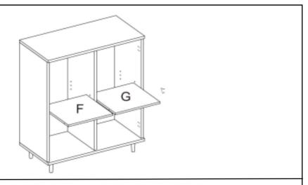
Put Left Adjustable Panel(F) and Right Adjustable Panel(G) on the Shelf Support(6)
