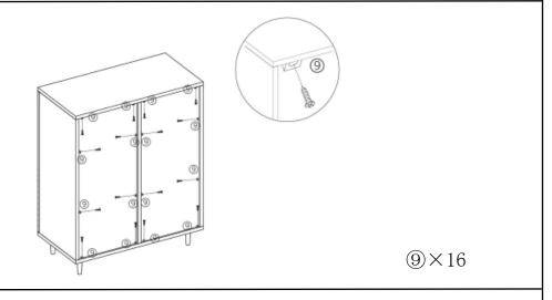
Attach Back Botton(9) to Back Panel(J) using AllenWrench(10).
