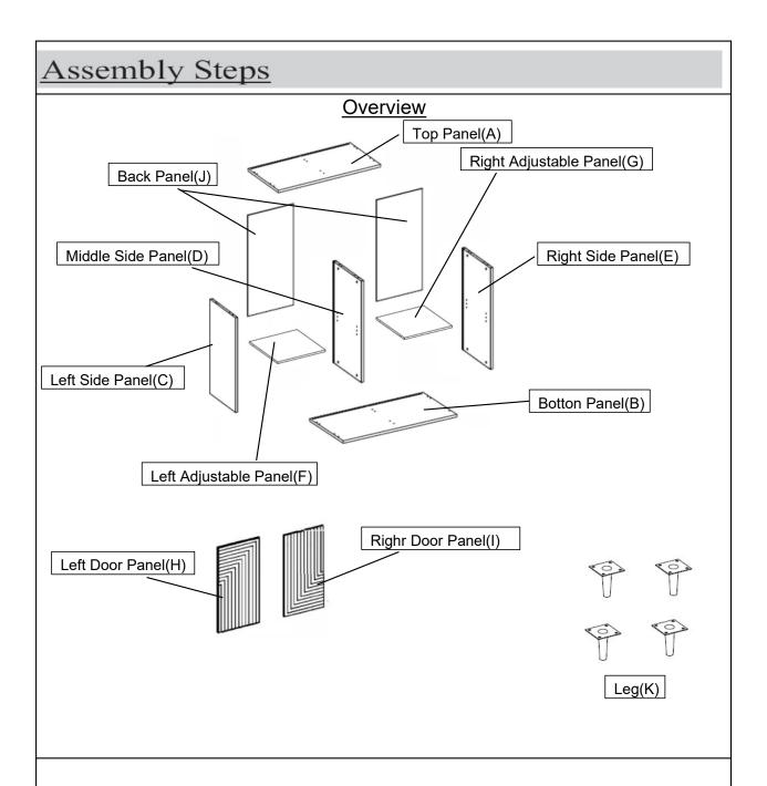
This <u>Cabinet</u> has multiple parts and may require up to some <u>60</u> minutes to assemble. To give you an overview of the <u>Cabinet</u> parts, the above picture is to help you put the various parts into perspective. Please read through the instructions below to familiarise yourself with the parts and steps before assembly.
