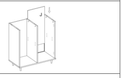
Insert another Back Panel(J) into the groove of Middle Side Panel(D) and Right Side Panel(E)
