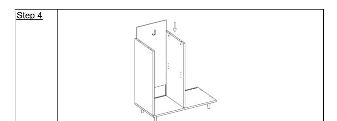
Insert Back Panel(J) into the groove of Left Side Panel(C) and Middle Side Panel(D).
