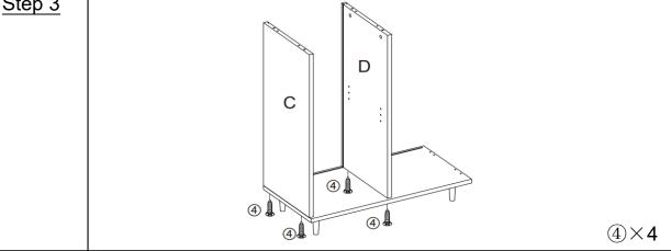
) into Left Side Panel(C) and Middle Side Panel(D) Insert Cam Nut( using Allen Wrench( ) turning anticlockwise until tight.
