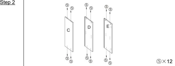
Attach the Dowel(5) to Left Side Panel(C). Repeat the previous steps to the Middle Side Panel(D), and Right Side Panel(E)
