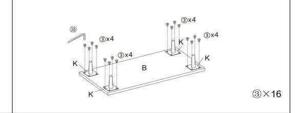
Attach the Leg(K) to Bottom Panel (B) with Bolt(3) using Allen Wrench(10).
