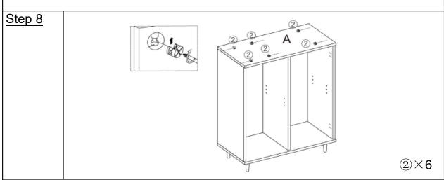
Insert Cam Nut(②) into the mounting positions on Top Panel(A) using Allen Wrench(⑩) turning clockwise until tight.
