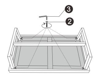
**STEP 2**: Connect both leg frames(B) with stretcher(C), lock with bolt (1) and allen key(3).
