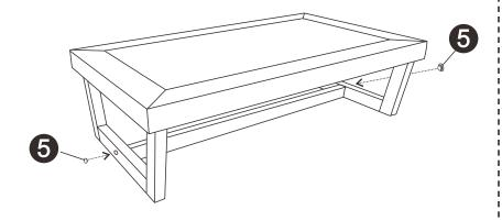
**STEP 4**: Cover the screw holes with plastic covers(5), assembly completed.
