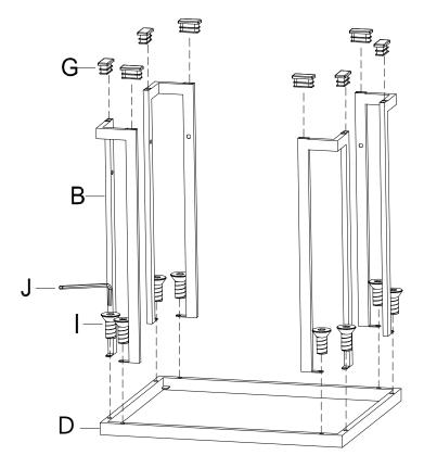
Attach the Bottom Frame (A) to the Leg (B) using Bolt (F) with the Allen Wrench (J).
