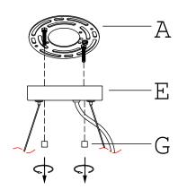
4 » Carefully pass supply wires through mounting plate
