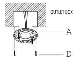
5 » If needed, shorten the length of fixture wires. At this point, the remaining wire length measured above canopy (E) is at least 6".
