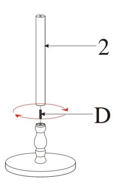
Screw the 60mm short screw (D) into the Base support rod (6),and then tighten and fix the Main circular rod (2) securely
