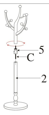
Firstly, screw the screw (C) into Main circular rod (2),insert the Central connecting piece (5), and finally tighten and securethe upper part
