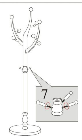
Finally, screw the Short rod (7) into the Central connecting piece (5) and tighten it securely
