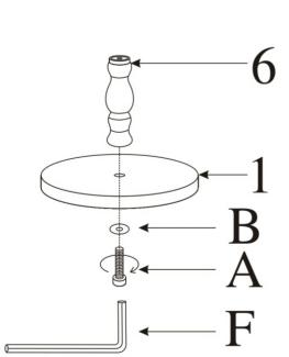
Install and connect the pedestal (1) and Base support rod (6) using screws A and washers (B), and finally tighten and secure with a Big wrench (F) 04
