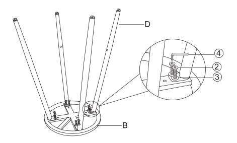
Attach the Leg(D) to the Cross Ring (B) using the Washer( $\Im$ ), Bolts( $\Im$ ) with Allen Wrench( $\Im$ ) as pictured above. Do not fully tighten the Bolts.
