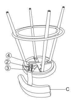
Attach the Leg with Ring to the Back(C) using the Washer (③), Bolts (③) with the Allen Wrench(④) as pictured above. Fully tighten the Bolts.
