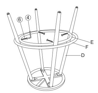
Attach Ring (E)and (F) to the Leg(D) using the Bolts (6) with the Allen Wrench (4).
