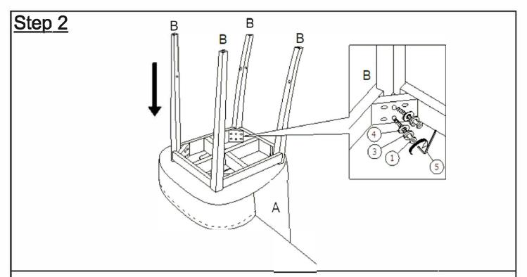
Place the Chair Seat(A) onto the side of a table as shown in the picture. Insert the Chair Legs(B) into the base of Chair Seat(A).
