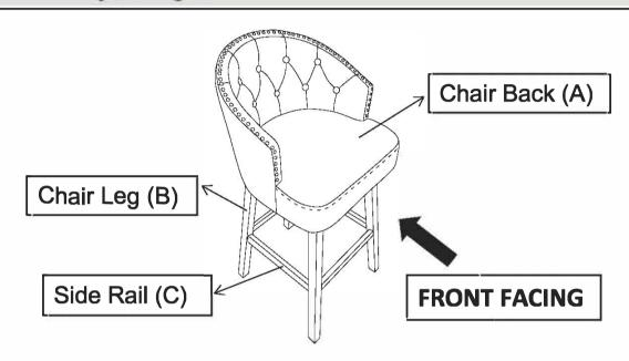
This Bar Chair has multiple parts and may require up to 30 minutes to assemble. To give you an overview of the Bar Chair parts, the above picture is to help you put the various Bar Chair parts into perspective. Please read through the instructions below to familiarise yourself with the parts and steps before assembly.
