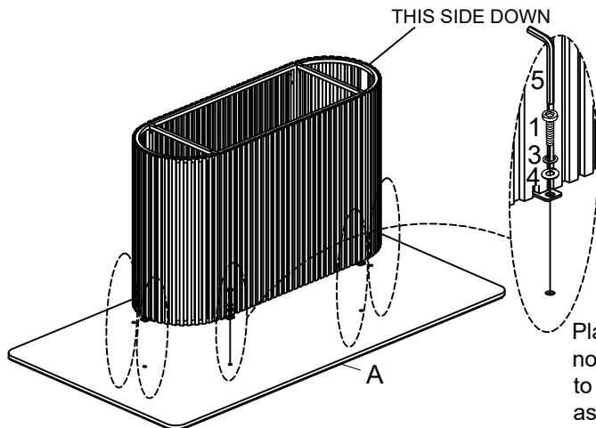
Place the tabletop facedown on a clean, non-marring surface. Attach the table base to the bottom of the tabletop using screws, as shown in the pictures.
