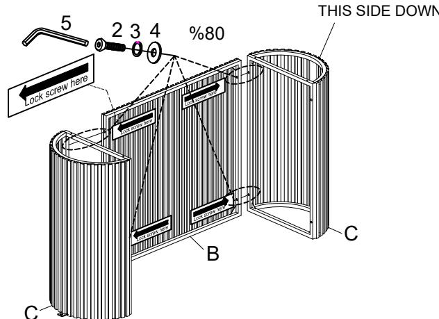
In this step, tighten the screws to 80%.
