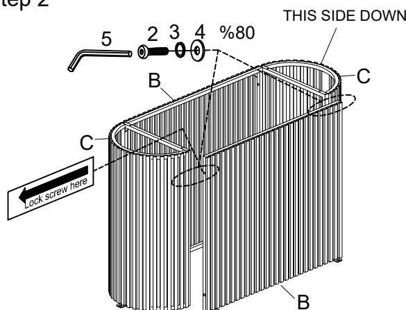
In this step, tighten the screws to 80%.
