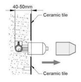
6.(2)Twist some Teflon tape on the adapter and screw it to the water pipe with big Allen key. Install the two fixed joints on both sides of the adapter as picture shows. Inset spout to the adapter then tighten it with screws.
