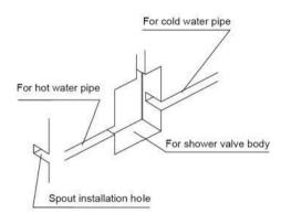
2.Recommended depth for installing shower valve body before tiling tiles: 40-50mm.Note:Tile opening should be bigger than shower valve diameter at least 5 mm.
