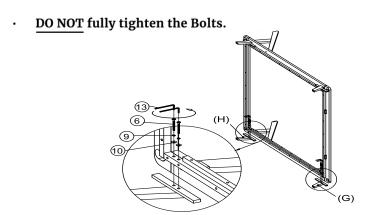
• With the help of your adult partner, attach the Second Support Bar (J) to the Headboard Bar (A) using Bolts (7), Spring Washer (9), Flat Washer (10) and the Allen Wrench (13) as shown below.
