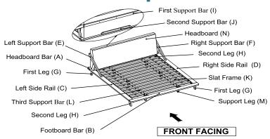
This Bed has multiple parts, and may require up to 45 minutes to assemble. To give you an overview of the Bed parts, the above picture is to help you put the various parts into perspective. Please read through the instructions below to familiarize yourself with the parts and steps before assembly.
